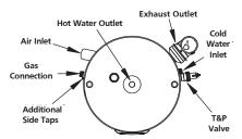
Top Outlet: 1" NPT Side Inlet: 1" NPT Side Taps: 1" NPT Condensate Drain Outlet: 1/2" NPT
