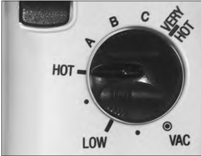
Figure 27 - Adjusting the gas control knob.
