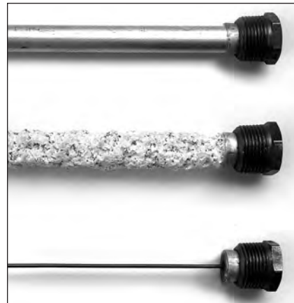
Figure 32 - Anode rods from new (top) to partially depleted (middle) to fully depleted stage (bottom).
