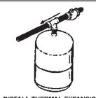
INSTALL THERMAL EXPANSION TANK IF WATER HEATER IS INSTALLED IN A CLOSED WATER SYSTEM.
