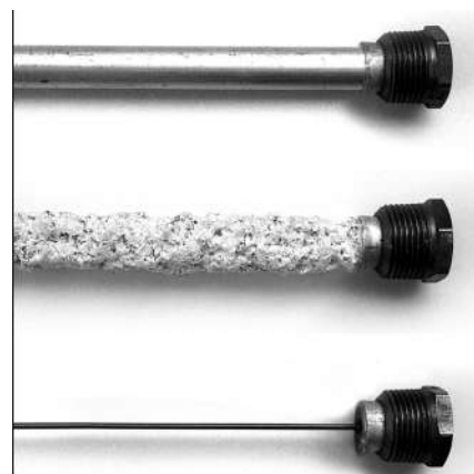
Figure 34 - Anode Rods from new (top) to partially depleted (middle) to fully depleted stages (bottom)
