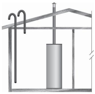
Figure 14. Outdoor Air Through Two Vertical Ducts
