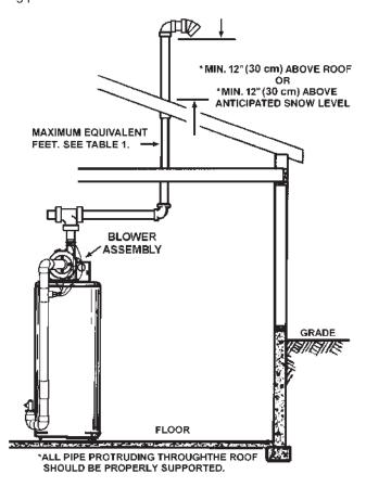
Figure 19. Through-the-Roof Vent Installation
