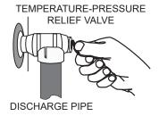
Figure 33. Testing the Temperature-Pressure Relief Valve
