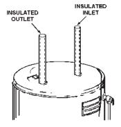
Figure 10. Cold and Hot Water Line Pipe Insulation
