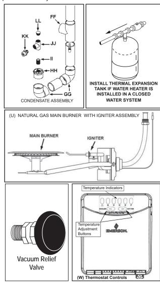
Figure 1. Features and Components - Right Side
