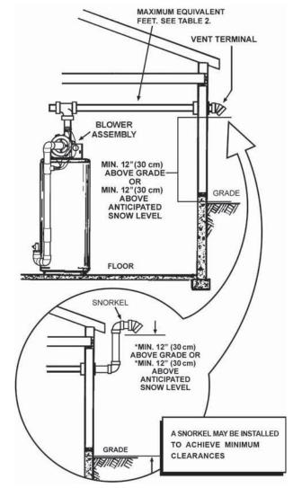
Figure 18. Sidewall Vent Installation
