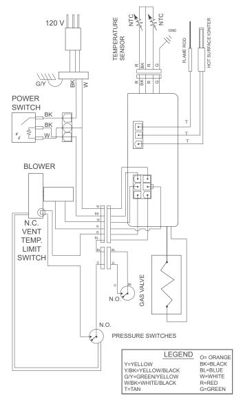
Figure 34. Wiring Schematic
