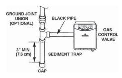
Figure 28. All Black Iron Pipe to the Gas Control Valve
