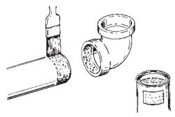
Figure 22. STEP E Applying Solvent Cement
