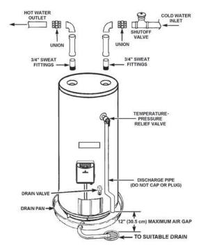
Figure 9. Typical Water Piping Configuration
