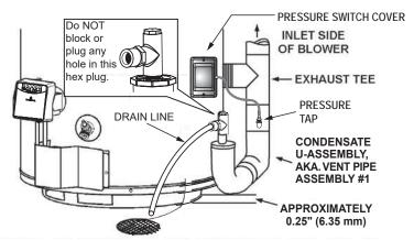
\*NO PORTION OF THE FIELD SUPPLIED DRAIN LINE BEYOND THE 1/2" ADAPTOR MAY BE ELEVATED HIGHER THAN THE ADAPTOR. THIS MUST BE TRUE FOR THE ENTIRE LENGTH OF DRAIN LINE INCLUDING EXIT INTO AN APPROPRIATE DRAIN.
