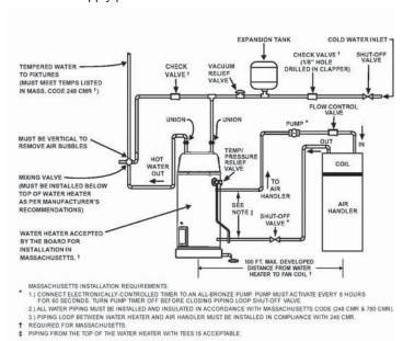
Figure 8. Space Heating and Potable Water with Mixing Valve
