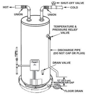
Figure 29. Typical Piping Configuration
