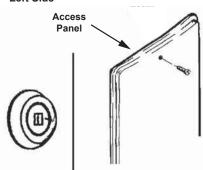
Caution: This access panel covers a 2" NPT plug that was required during the manufacturing of this water heater. This 2" NPT flange is not a cleanout fitting, removing the 2" NPT plug and using this fitting as a cleanout could void your warranty.
