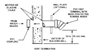
Figure 17. Sidewall Vent Termination
