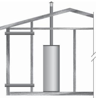
Figure 13. Outdoor Air Through Two Horizontal Ducts
