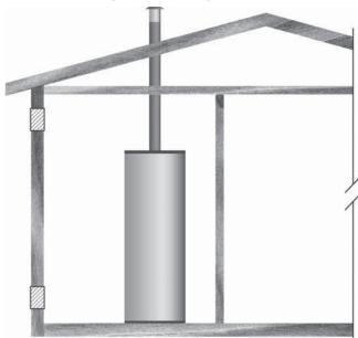
Figure 11. Outdoor Air Through Two Openings
