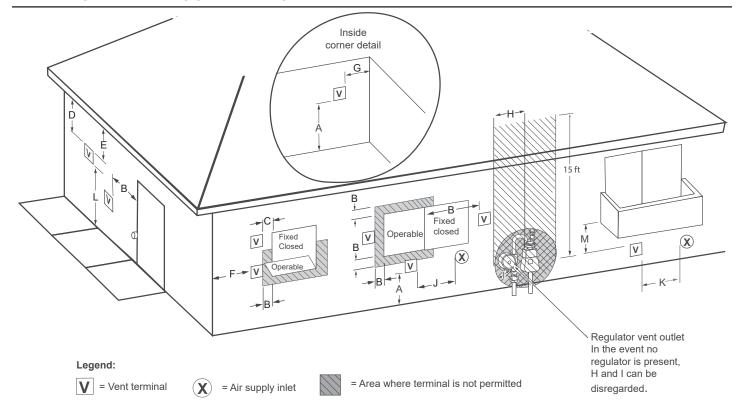
Figure 25. Other than Direct Vent Using Outside Air
