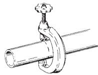
Figure 20. STEP A Tube Cutter for Cutting Plastic Pipe
