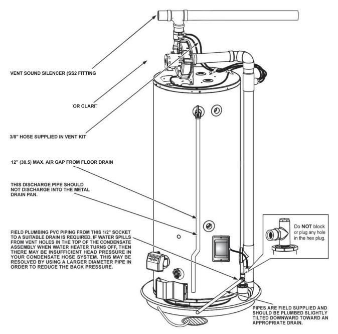
Figure 2. Features and Components - Left Side
