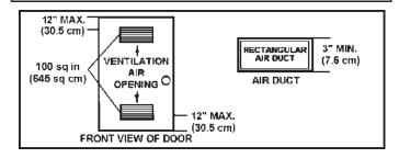
Figure 7. Combustion Air and Ventilation Requirments
