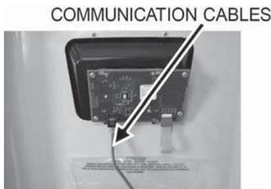
**Figure 27. Locating the Communications Cable on Back of the Display**
