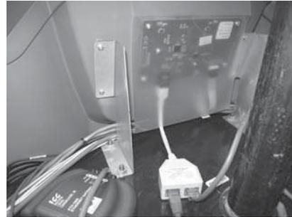
**Figure 23. Reconnecting the Communication cord to the Receptacle**
