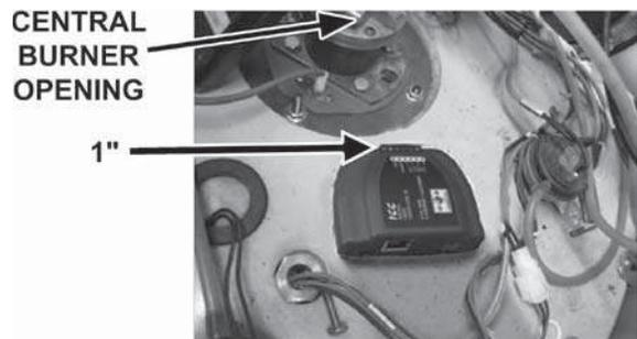
**Figure 25. Connecting the Communications Cable to the Module**
