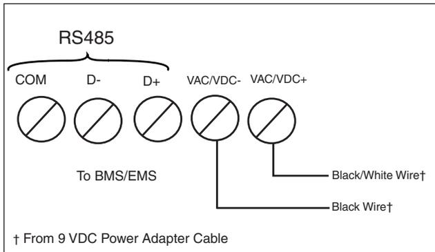
Figure 11. Port A Connection Diagram
