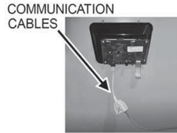
**Figure 29. Connecting the Display Cable to Split Cable Receptacle**
