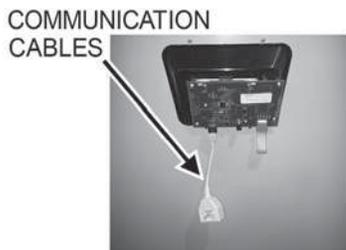
**Figure 28. Reconnecting RJ45 Plug from Split Communication Cable**
