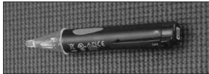
Figure 21 - Use a non-contact circuit tester to check for electrical power.
