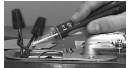
Figure 32 - Non-Contact Circuit Tester
