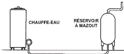
INSTALLATION AVEC CONDUITE D'ALIMENTATION SEULEMENT ET ÉCOULEMENT PAR GRAVITÉ - FIGURE 11
