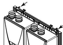
**Figure 2: Spreader Lifting Bar**
